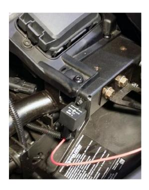
6. Connect power wire to horn from relay. Using the image below, run your red wire with the 1/4" terminal to the horn. Do not secure the wires at this time.
