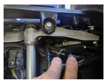
3. Push the rubber cover back and remove the dead plug from the connector. Plug in your new harness. Place the rubber boot back into it's original location. Run the harness under any part of the frame over to the battery area.
