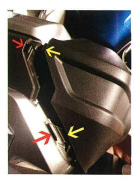
24. Secure the cowl by inserting and tightening the screws shown by the yellow arrows.
