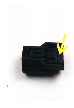
8. The short leg of the harness goes to the right light. Bring it up to where you can access it and plug the light into the harness. Red to red and black to black. Run the long leg to the left light behind the lower cowl and connect. Use supplied wire ties to secure the wire as needed.
