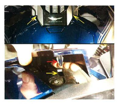
10. Use your 5mm allen wrench to remove the screw shown by the yellow arrow. You will have to remove the push pin shown by the red arrow. Pull on the center of the head until it pops up and then pull it out of its hole. (R)
