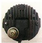
Note: to reinstall the push fasteners, do the following before inserting into the hole. Hold the base of the fastener while you push up on the center of the pin. Once it is pushed up, insert the fastener into the hole.
