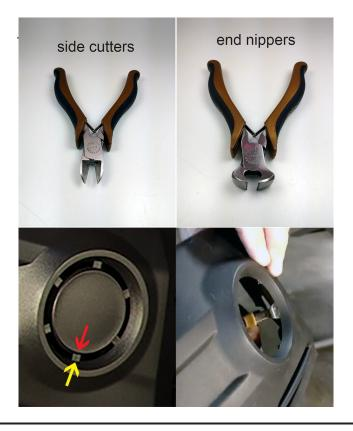
9. Mount the light to the bike using the bolt you removed in step 3. Position the bolt in the center of the slot as shown in the insert pic with yellow arrow. Use your wrench to tighten the bolt so that the light is held in place. We will need to adjust the side to side position of the light behind the hole in the cowl, so don't overtighten the bolt. (R)
