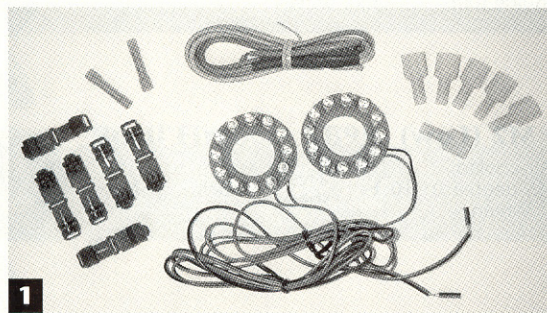
1 This is The Electrical Connection's rear turn signal conversion kit. Simple as it looks, it works very well.
